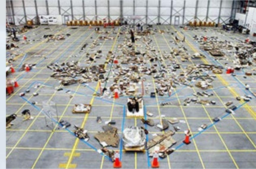
Debris from the fallen space shuttle Columbia as seen in May 2003 during a reconstruction effort as part of the accident investigation. The debris was later moved into the preservation office. (NASA)
