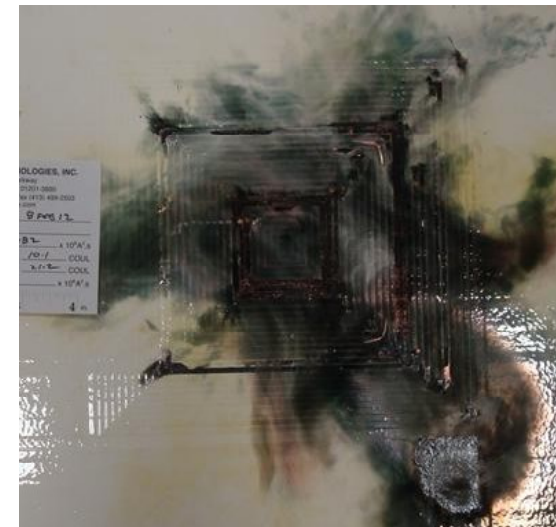
Post Strike Damage
