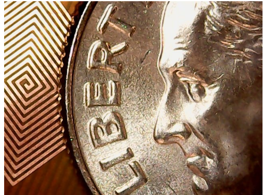
.15 mm trace width using conventional etching printed circuit board manufacturing techniques
