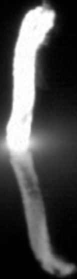
High Speed Video First Frame showing Lightning Strike Initial Attachment on Mesh Protected Carbon Panel
