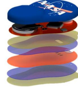
AstroSense wireless wearable sensor (cortisol, temp, humidity)
