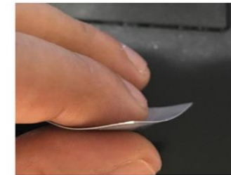
Flexible, printed supercapacitor for energy storage
