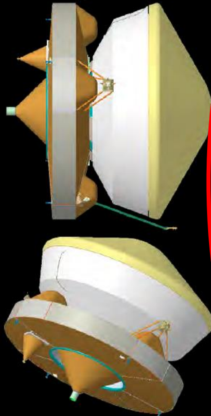
Spacecraft = Cruise Stage + Entry Vehicle
