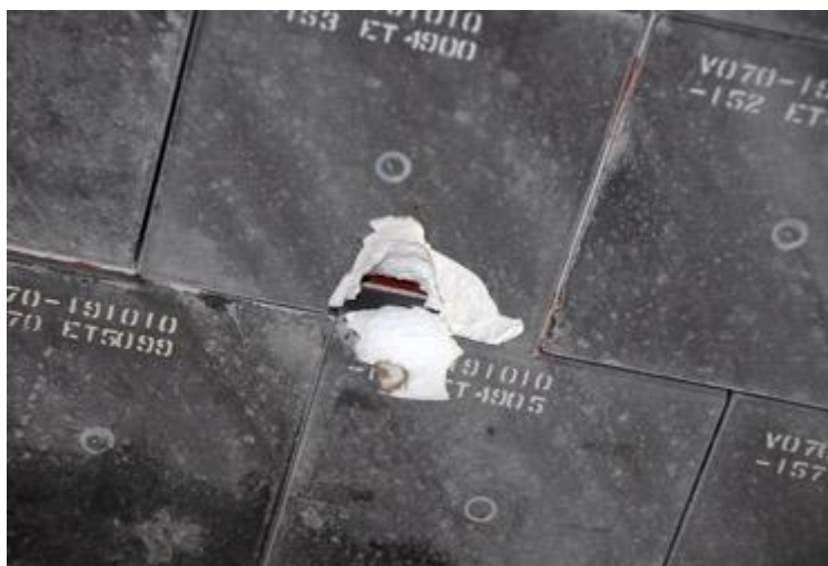
On-orbit tile damage inspection
