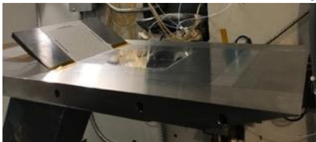
Flat Plate Model with Wedge in 20 M6 Tunnel
