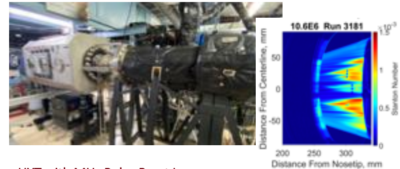
HXT with MHz Pulse Burst Laser (Limbach and Bowersox)
