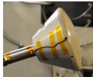
Orion blocked heatshield model, made of PEEK material, in LaRC Mach 6 Tunnel
