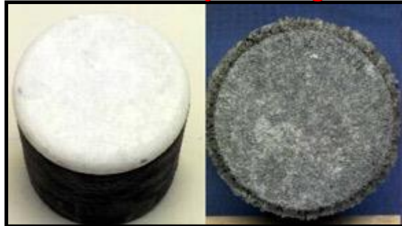
TPS material before and after arc-jet testing
