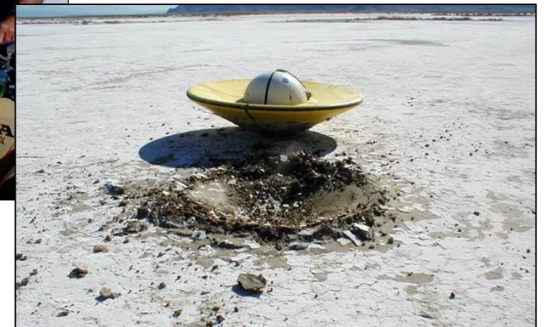
Drop Testing of the First EEV Prototype at the Utah Test & Training Range (UTTR) in 2000
