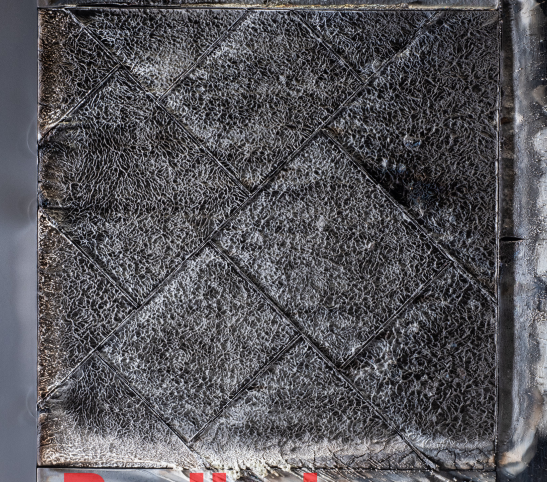
Heat Shield Avcoat Block/Seam Array in Combined Convective/Radiant Heating
