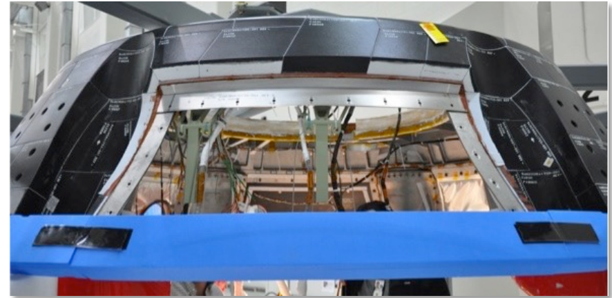
Forward Bay Cover, with Side Panel Removal
