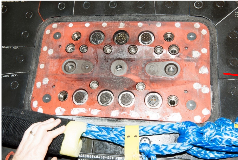
Charring of RTV on Umbilical Panel
