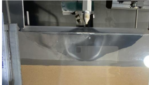
BP-1 crater generated under near-vacuum ambient pressure during pathfinding site visit work
