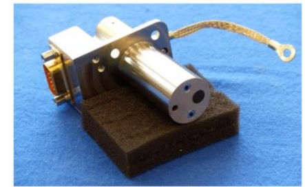
(Aerothermal sensors used for ExoMars)
