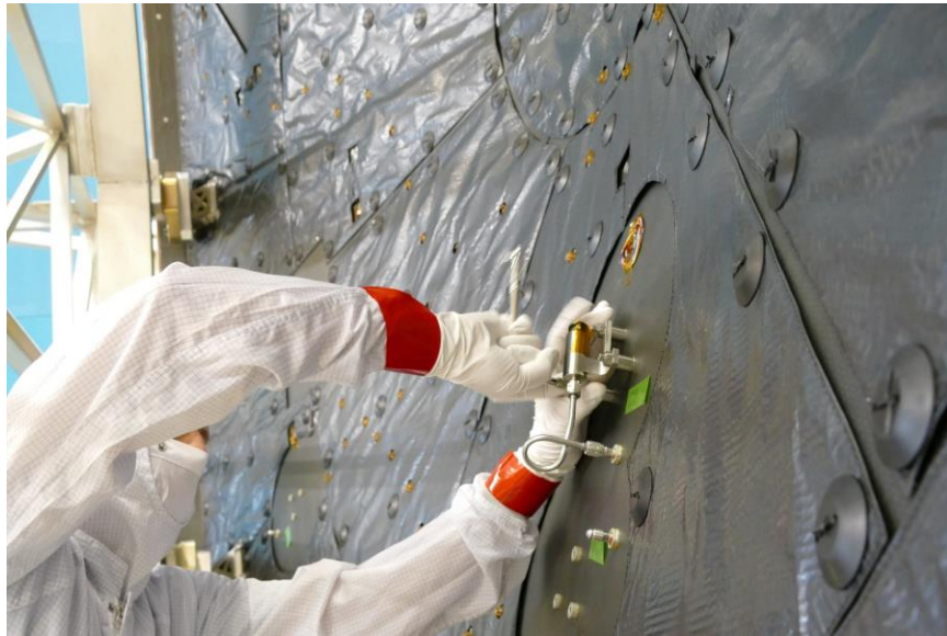
MEDLI2 pressure transducer installation
