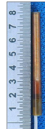
Hollow aErothermal Ablation and Temperature (HEAT) sensor
