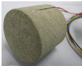
(Thermal plugs used for MEDLI2)
