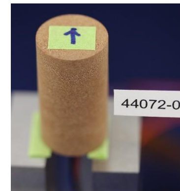
Artemis 2 Heat Shield Thermocouple (TC) plug
