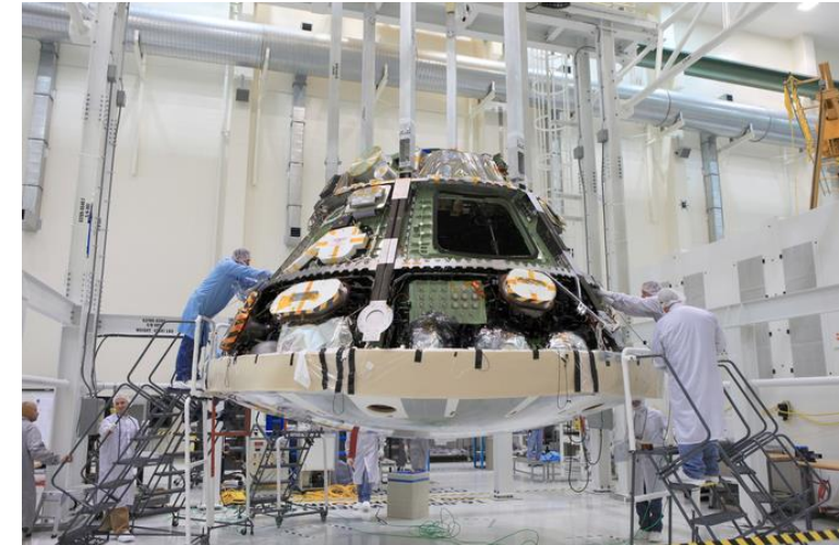
Heat Shield Installed
