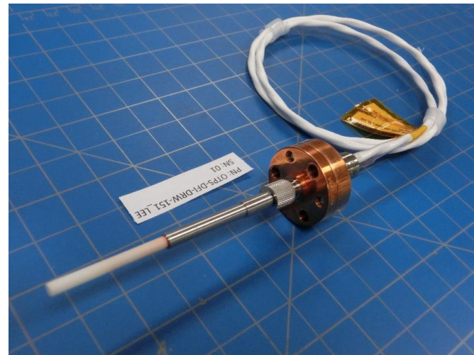
Heat shield radiometer
