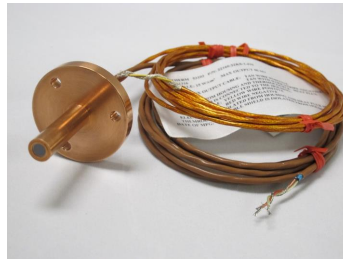
MEDLI2 Backshell Radiometer
