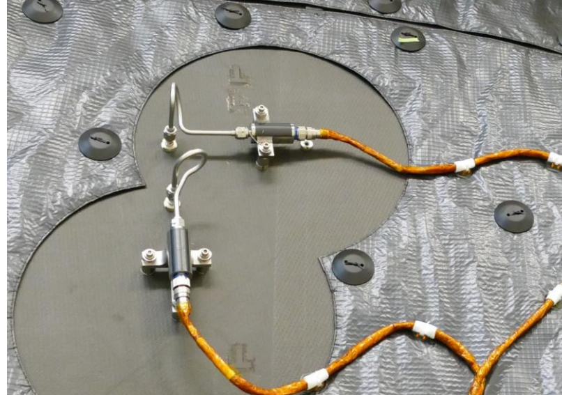
MEDLI2 Hypersonic and Supersonic pressure transducers installed on the Mars 2020 heat shield
