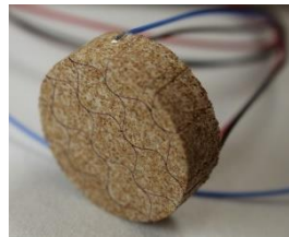
(Thermal plugs used for MEDLI2)
