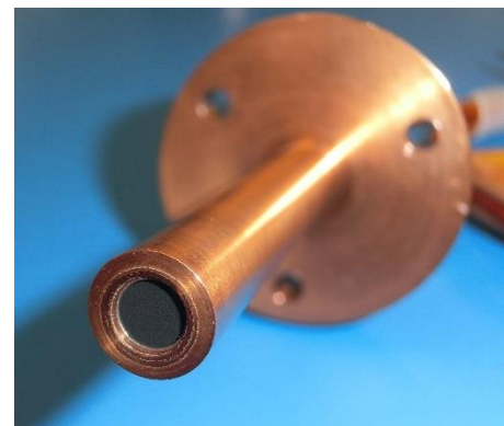
Artemis 2 Backshell Radiometer
