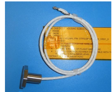
Artemis 2 Heat Shield Optical Recession Sensor (ORS) – plug and diode housing
