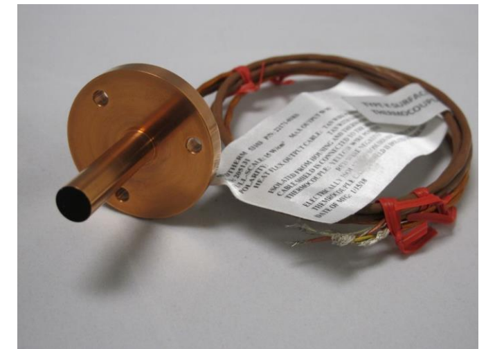
MEDLI2 Backshell Total Heat Flux Sensor
