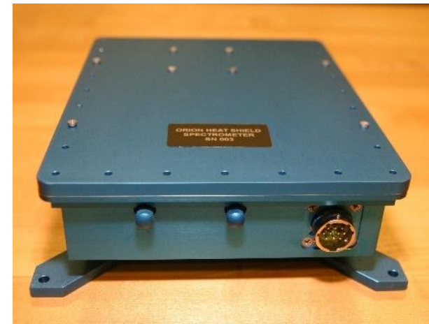
Images of Artemis 2 spectrometer housing (development unit) 12
