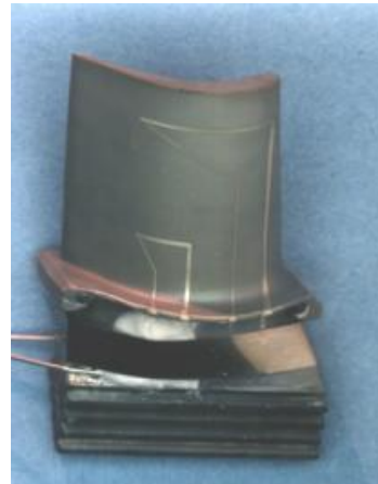
Pt- Pt/Rh temperature sensor to T=1200^{\circ}\text{C}
