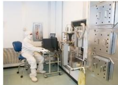
Oxidation and Annealing Furnaces and Silicon Dioxide Low Pressure Chemical Vapor Deposition System
