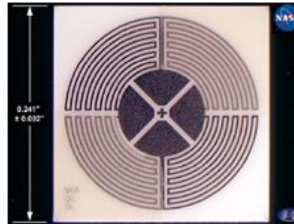
Heat Flux Sensor Array to T=1000^{\circ}\text{C}
