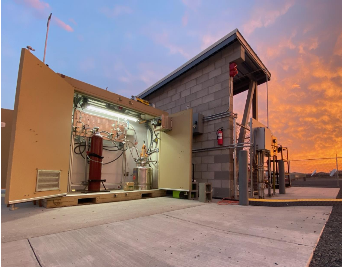
WSU's deployable hydrogen liquefier (photo credit Leif Harfst)
