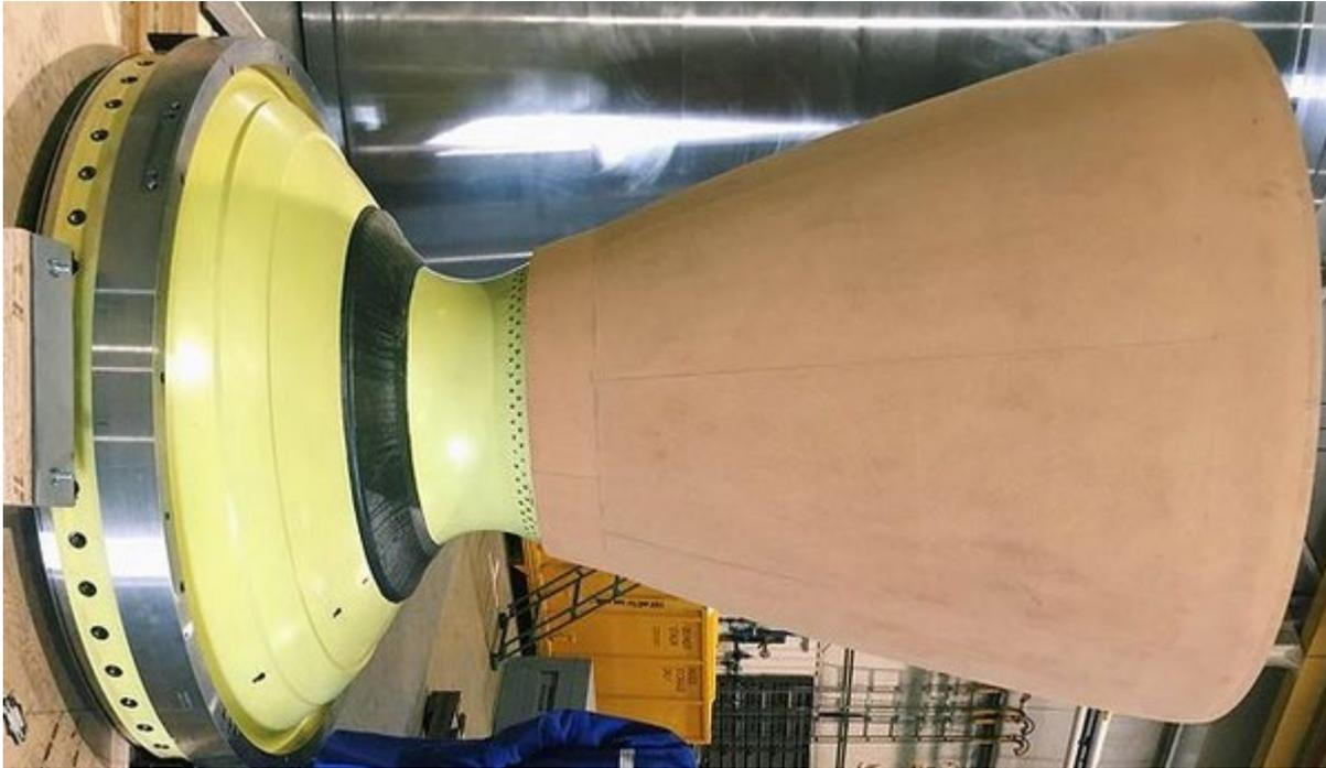
Figure 1: Typical SRM Nozzle
