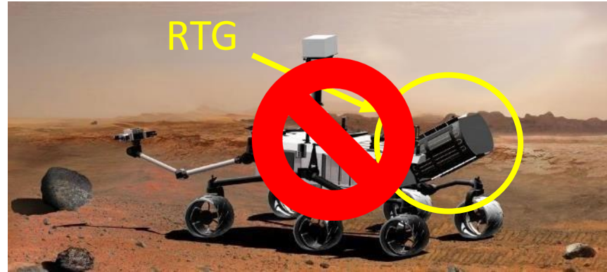
Radioisotope thermoelectric generator (RTG) of Curiosity rover
