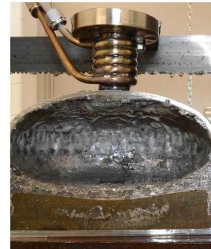
Cross-sectioning and CT scan of the reactor
