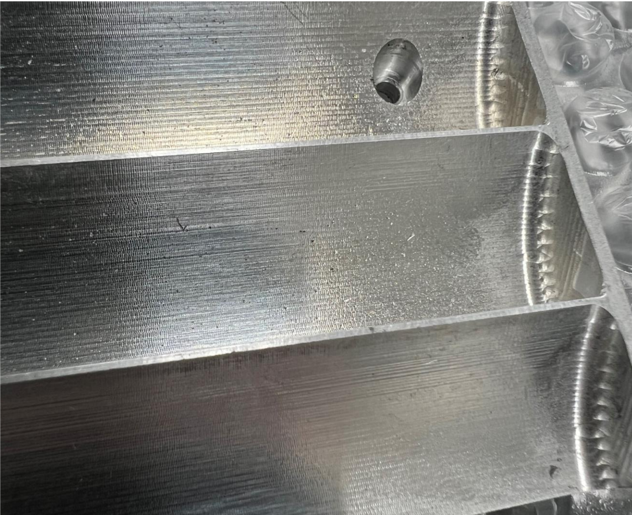
Completed PRR Reflector: Unpolished Surfaces
