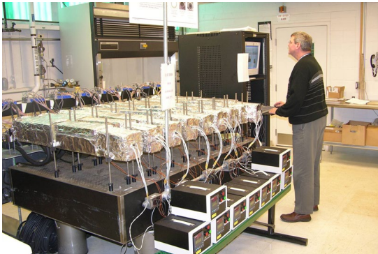
CP 2 Titanium-Water Life Test with 50,000 Hrs. Ref. NASA/CR-2007-214820
