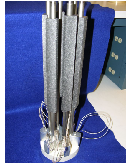
Titanium-Water Thermosyphon Gamma Radiation Exposure NASA/TM—2012-217732 AIAA-2012-4078
