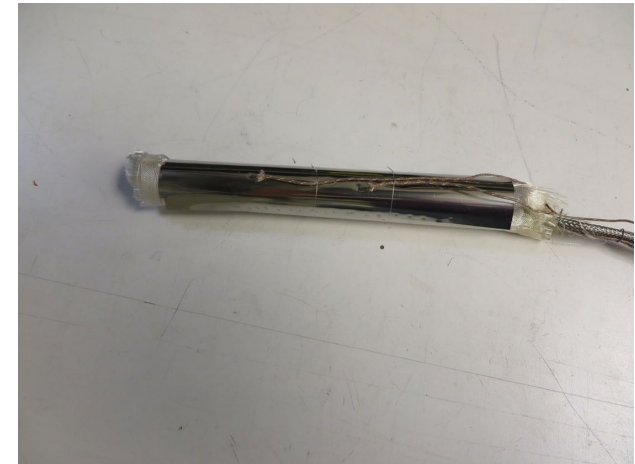
Instrumented 600 W heater with 5 layers of SS foil with quartz fabric
