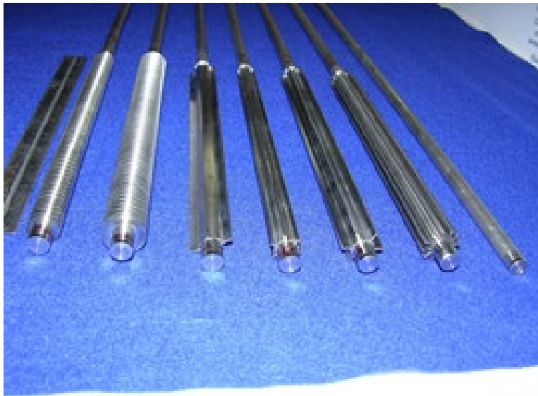
Titanium water thermosyphons with enhanced surface area
