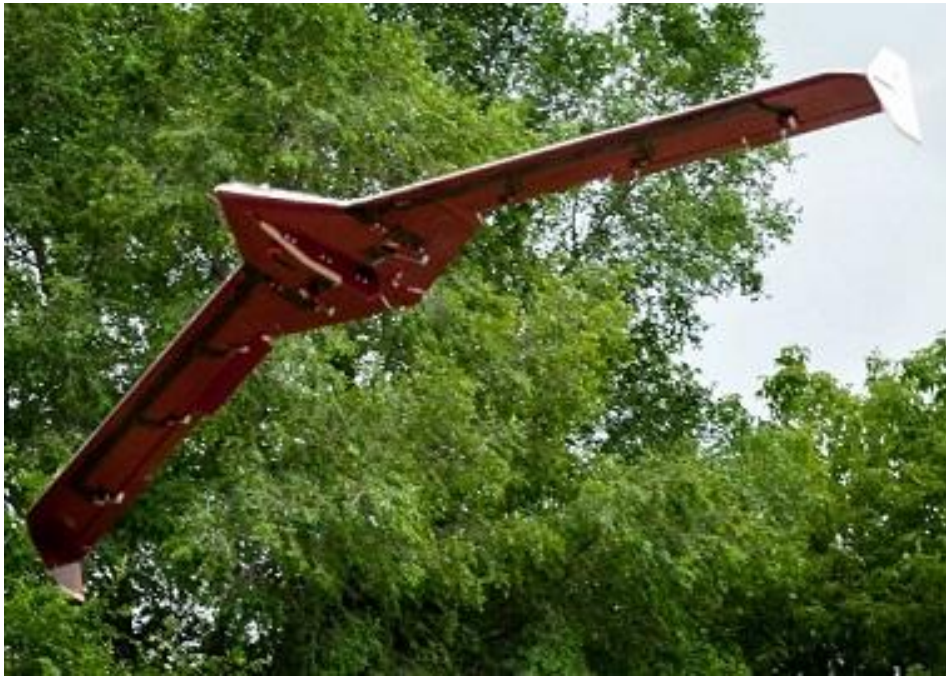
mAEWing1: BFF Replica 10ft wingspan, 14lbs
