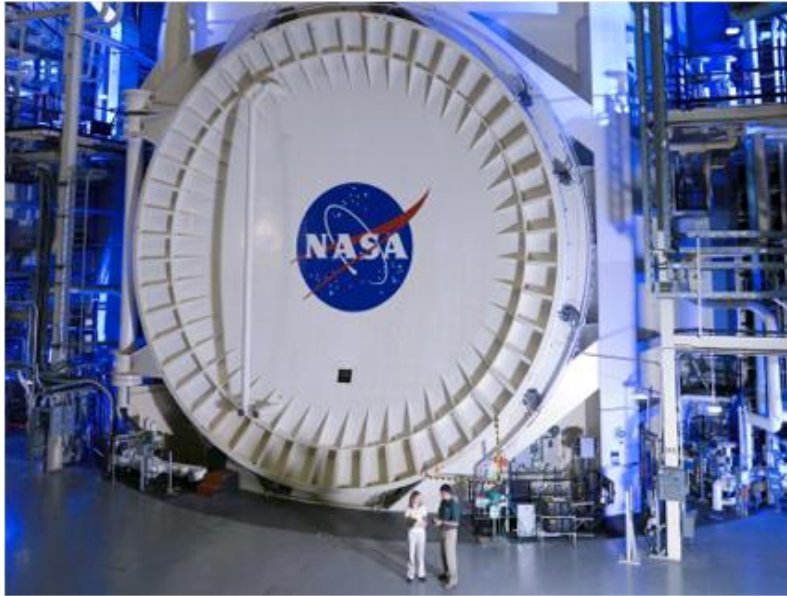
NASA Thermal Vacuum Chamber at Johnson Space Center Photo courtesy of NASA ( www.nasa.gov )
