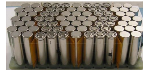
Li-Ion battery cells [Image courtesy of NASA]
