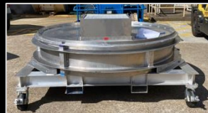
Regolith bin for PSI testing (~2m diameter)
