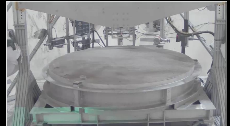
Regolith bin for PSI testing (~2m diameter, ~1700 kg of simulant per test)
