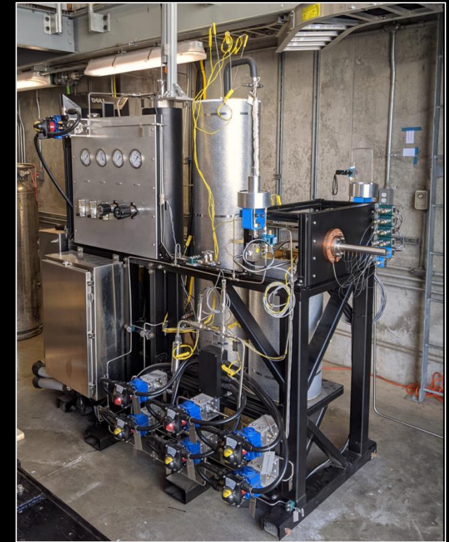
Ethane Supply Skid (External) (Purdue Univ. / NASA SSC)
