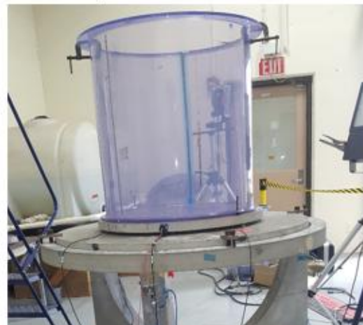
Slosh Test Fixture Cylindrical Tank Installed
