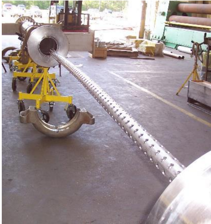
A long cylindrical capacitance liquid level gauge being installed.
