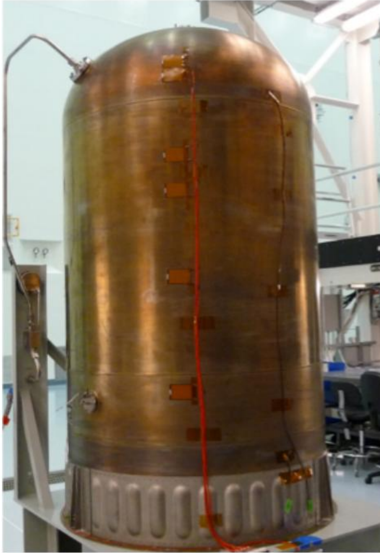
A Space Shuttle Orbital Maneuvering System Propellant Tank with 8 sensors installed.
