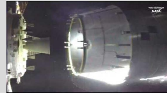
Fig. 1 Command module/service module separation.
