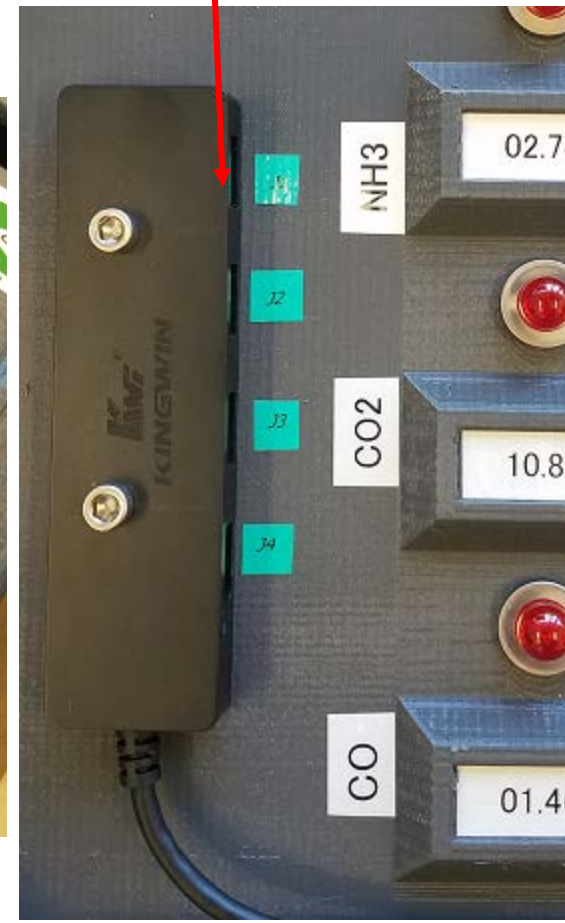
Sideways installed connectors complicate installation
