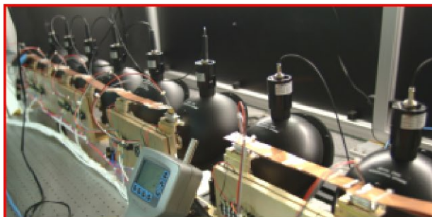
Fully automated custom vacuum chamber with 12 LDA test positions & windows for continuous inspection
