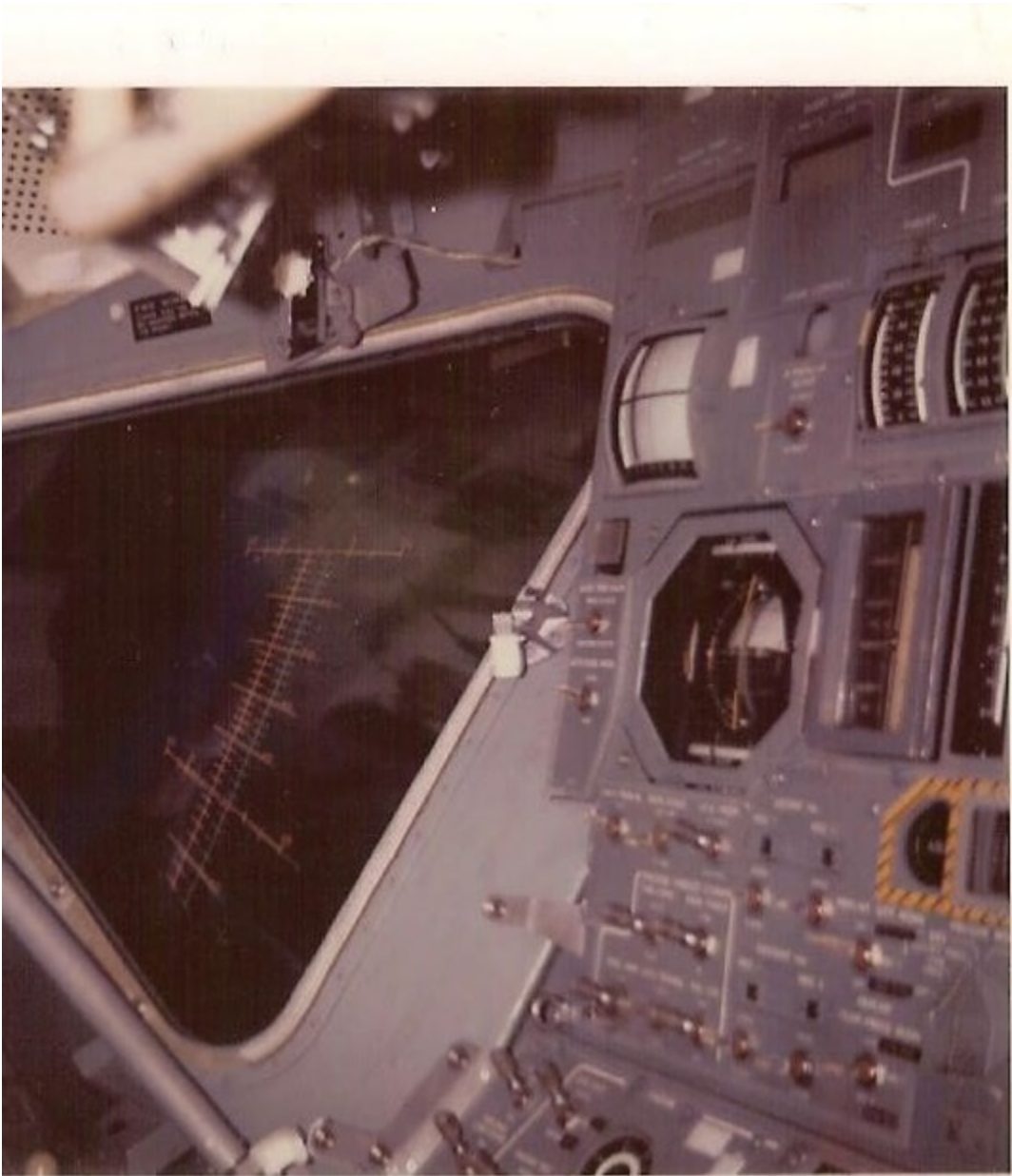
FIGURE 7. LM LANDING POINT DESIGNATOR (LPD)
