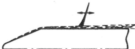
Shock Wave Oscillation with Attached Flow
