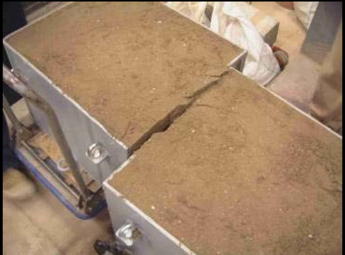
Laboratory scale modeling of strike slip faulting
