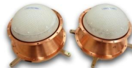
REBR (2) H-IIB 4.5 kilograms with heat shield
