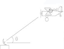
Given a ground station tracking an airplane, moving in a straight line at a constant speed, with only bearing measurements, we are interested in knowing the speed of the airplane and its position at the beginning of the tracking pass  $(x_0, y_0, u_0, v_0)$ . The equations are
