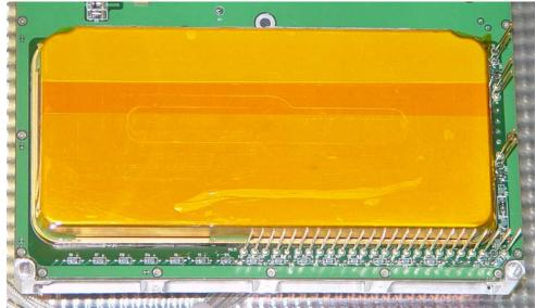
ULTEM is readily gold plated making it especially useful in applications where triple-junctions must be avoided. This cover is also covered with Kapton tape.
