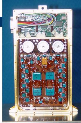
Note the holes in the PC board to improve penetration and bubble removal. Plastic nuts are also removed on spacers to allow board to float in the potting.
