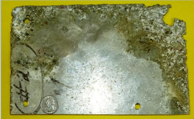
Corroded Al Plate (Front)
