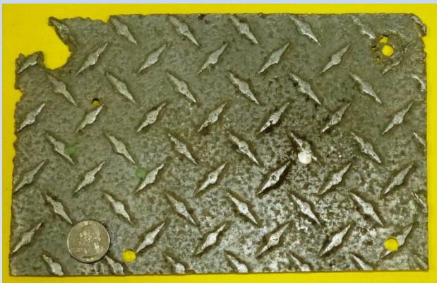
Corroded Al Plate (Back)
