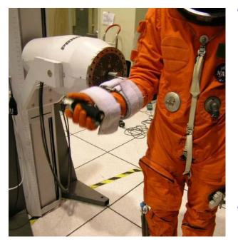
The test setup required a manned suit to be attached to the Primus RS<sup>™</sup>, the subject then set their own comfortable ROM, then the subject remained passive while the Primus RS<sup>™</sup> moved them through the ROM while calculating the torque.
