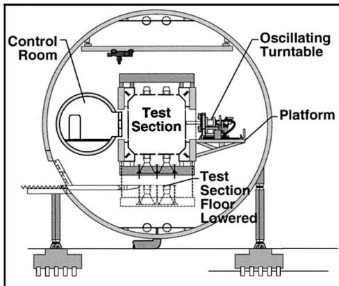
Fig. 1 Cross section of TDT showing test section and location of OTT.
