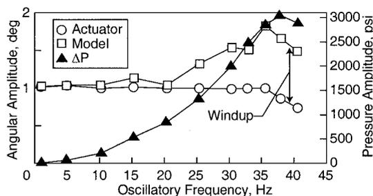
**Fig. 5** OTT performance data with inertia model.
