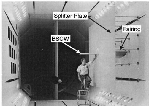
Fig. 8 BSCW model mounted in TDT test section.
