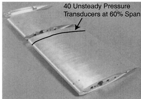
Fig. 7 BSCW model (disassembled) with transducer locations highlighted.
