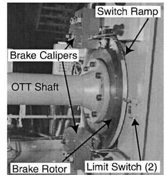
Fig. 3 OTT brake components.
