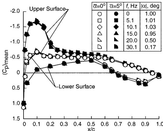
Fig. 11 BSCW mean pressure coefficients for  $\alpha = 0$  and  $5$  deg at  $M = 0.7, Q = 170$  psf, and  $Re = 4.53 \times 10^6$ .
