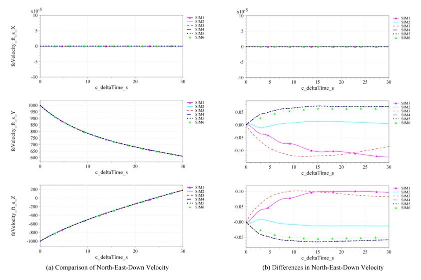
Figure 5. Atmospheric Scenario 9 Results for North-East-Down Velocity
