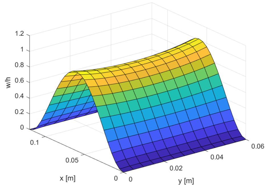
Static displacements due to static uniform load
