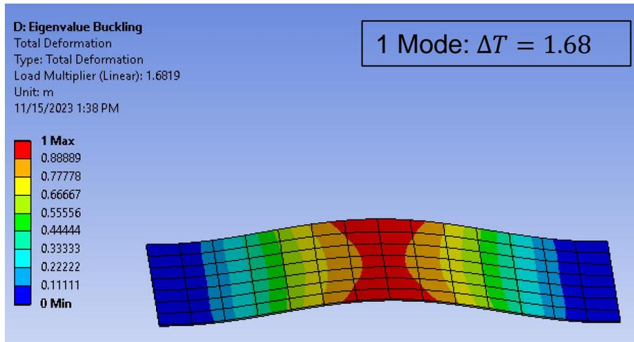
The thin ( $h = 0.406mm$ ) panel will buckle for  $\Delta T \geq 1.68$
