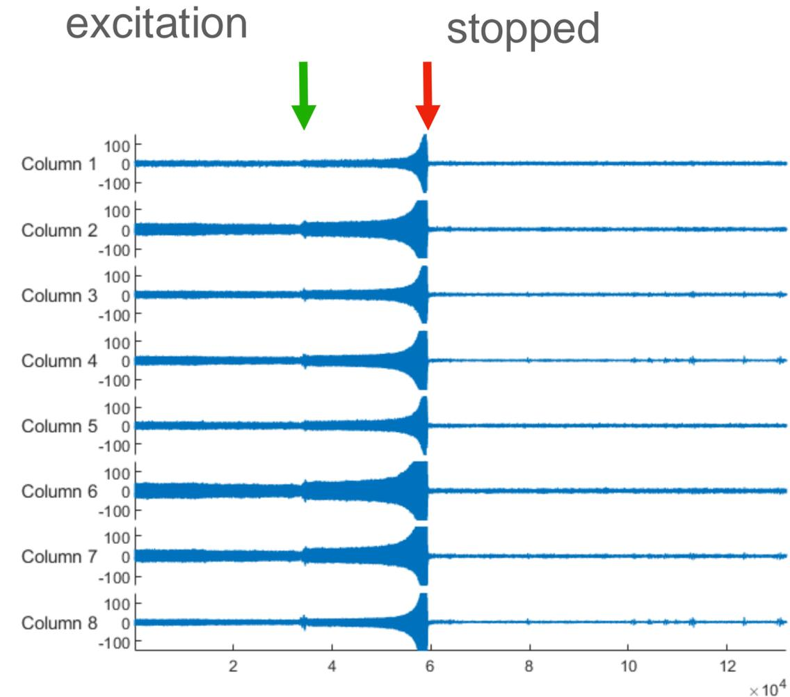
The wind tunnel turbulence is not sufficient to trigger the flutter onset at this specific dynamic pressure. A smaller perturbation are introduced in correspondence with the green arrow and slowly evolves either into rapidly increasing oscillations or towards the trivial solution.
