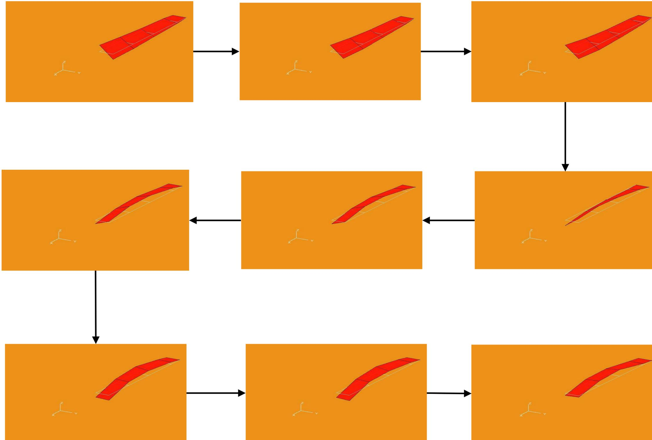
The 1st torsional mode becomes a flexo-torsional, decreasing the frequency at increasing values of velocity
