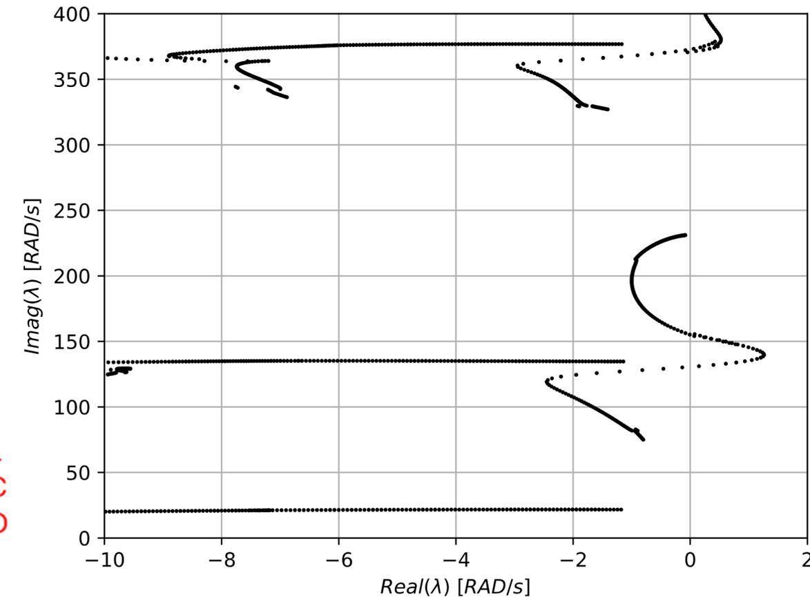
Good agreement between numerical and experimental results. The second instability is observable in both root loci. A fifth mode is excited and move towards the imaginary axis. LCO points with a value of damping close to zero are plotted.
