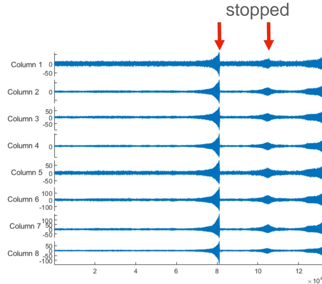
The wind tunnel turbulence is sufficient to trigger the flutter onset at this specific dynamic pressure. From the analysis of the signal, we notice that the system is unstable, develops rapidly increasing oscillations
