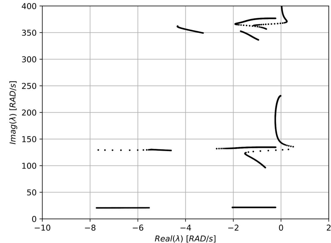
The fifth flexural-torsional mode is evident. This mode is probably not properly excited for low angles of attack.
