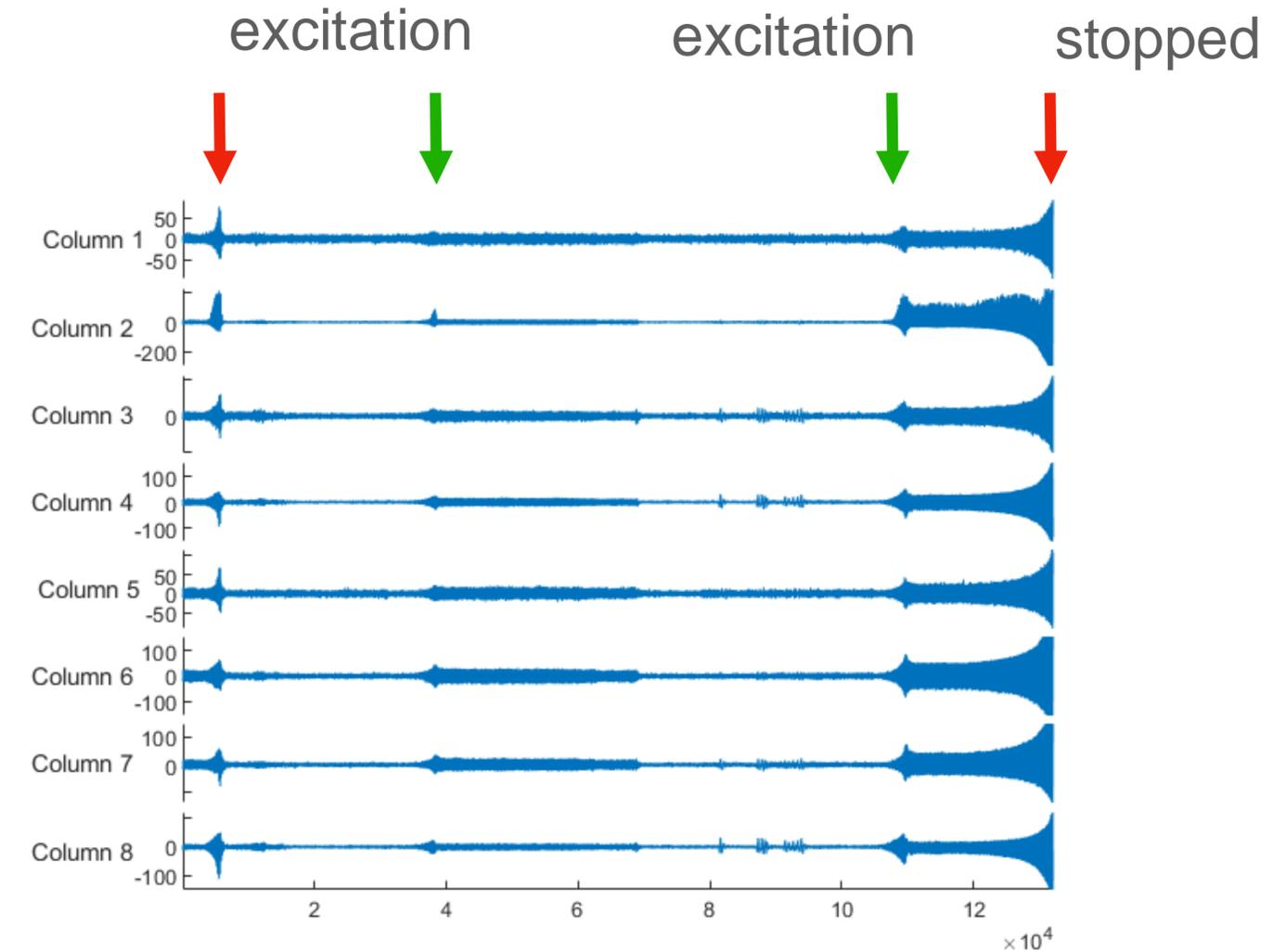
The wind tunnel turbulence is not sufficient to trigger the flutter onset at this specific dynamic pressure. A smaller perturbation are introduced in correspondence with the green arrow and slowly evolves either into rapidly increasing oscillations or towards the trivial solution.
