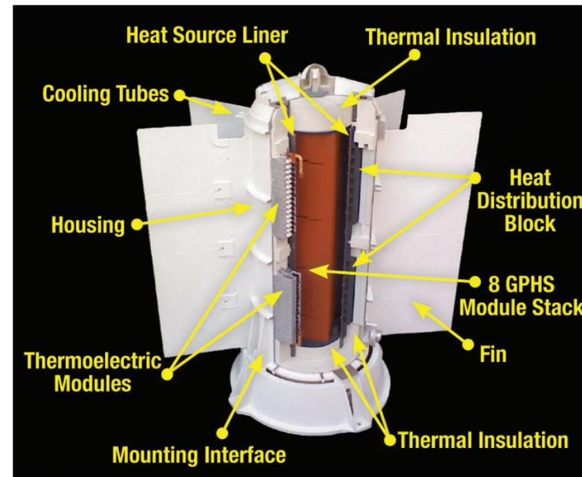
Cutaway View of an MMRTG
