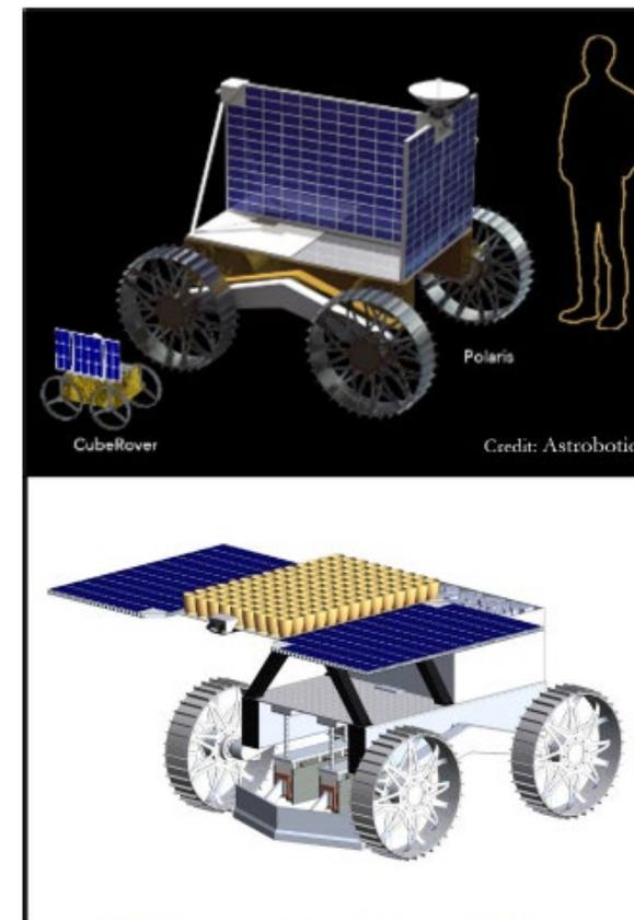
Figure 17. Upper: Astrobotic Polaris and CubeRover. Lower: Polaris reconfigured for *FarView* with VDM payload and solar concentrators.
