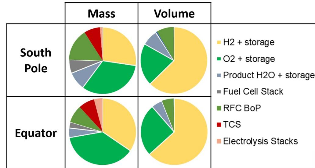
10 kW Class RFC system using 1500 psia reactant storage
