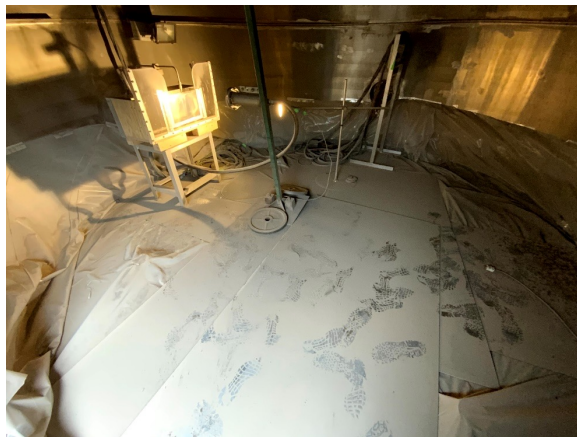
BP-1 dust coating over entire 15-foot vacuum chamber after pump-down outgassing and erosion during pathfinder testing in Jan. 2021
