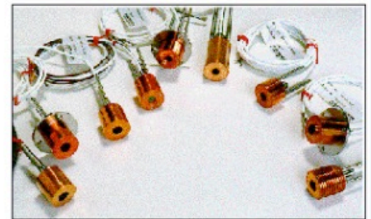
Lander base instrumentation (heat flux, pressure, other)
