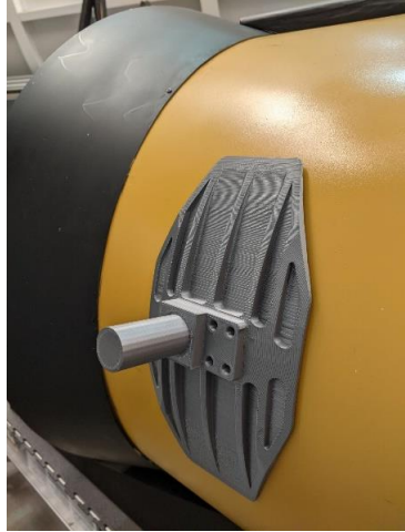
MAV SRM-1 to Vector Trunnion Pin
