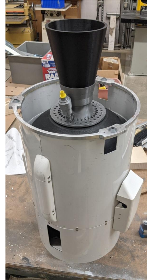
MAV SRM2 with Nozzle and igniters
