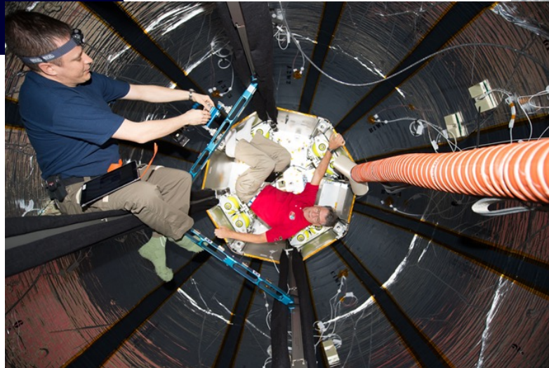
BEAM view with sensors installed on air barrier prior to stowage configuration
