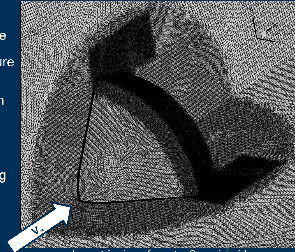
Isometric view of quarter Genesis grid
