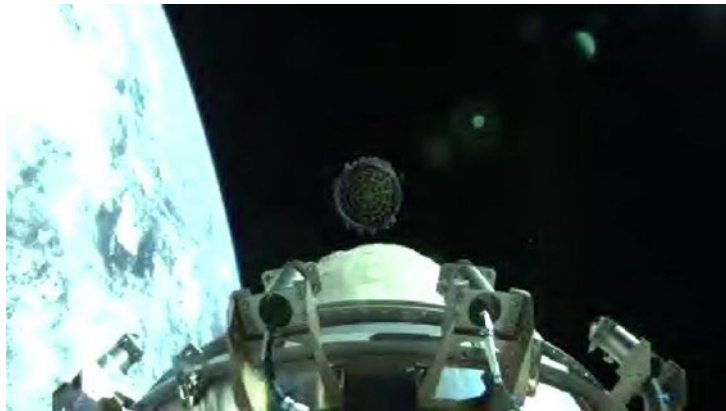
Novel long-stroke Payload Adapter Separation System (PASS)
